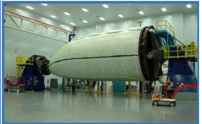
Line #6 C Axis Leak Check
